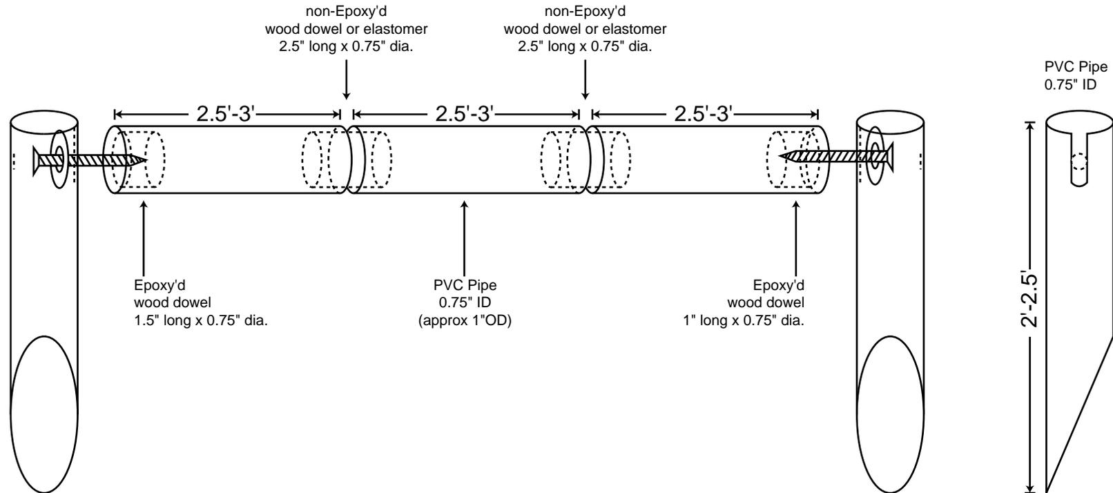
1. Cut 3 sections of 0.75 ID PVC pipe at 2.5'-3' for barrier crossbar.
